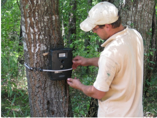
A trail camera records the times and dates as well as the number of pigs visiting a bait site.
