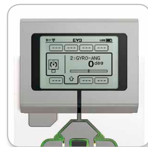
Port View with Gyro Sensor
